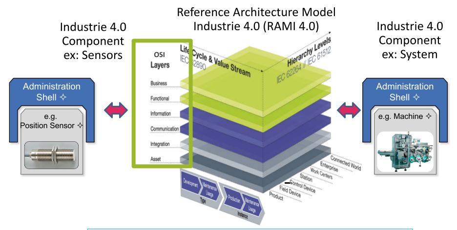
RAMI 4.0 – A Standards-based Architecture to enable connectivity between Industrie 4.0 Components
