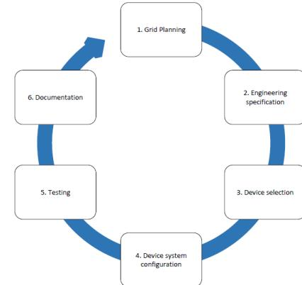
Fig. 3 Digital Substation Design Process
