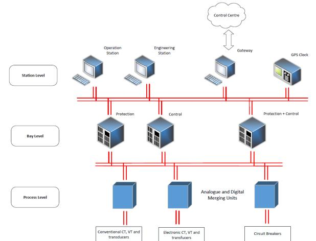
Fig. 4 Digital Substation Layout
