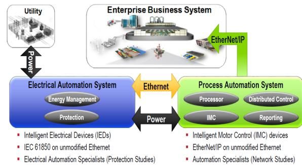
Fig. 2 Network Incorporating Electrical and Process Automation Systems
