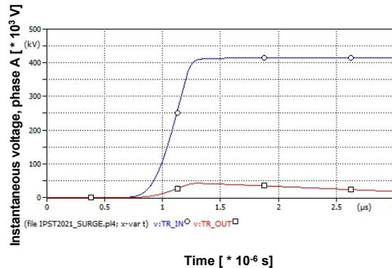
Fig. 4 Lightning overvoltages on 220 kV and 11 kV transformer windings
