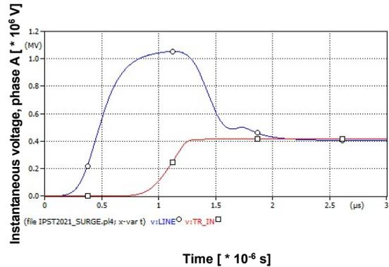
Fig. 3 Lightning overvoltages on 220 kV side (line and transformer)
