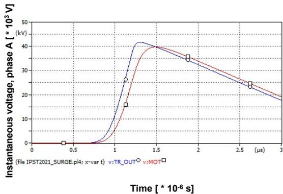
Fig. 5 Lightning overvoltages on transformer and motor 11 kV windings
