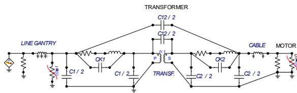
Fig. 2 EMTP-ATP model of the electrical system
