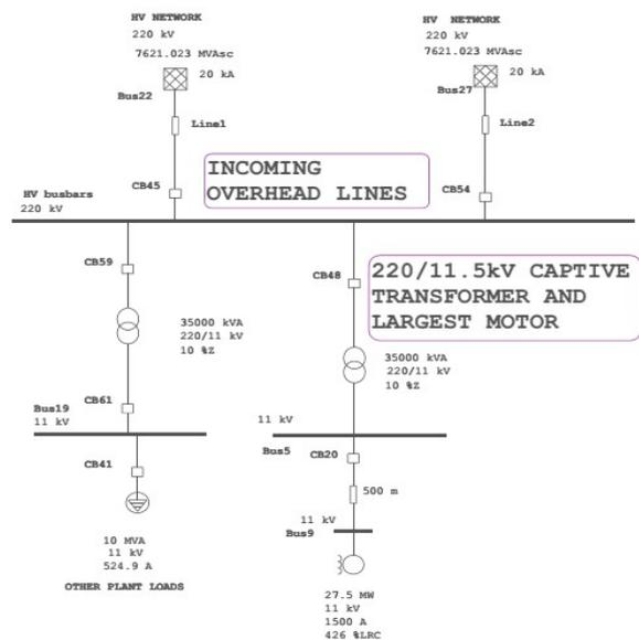
Fig. 1 Single-line diagram of the industrial electrical system
