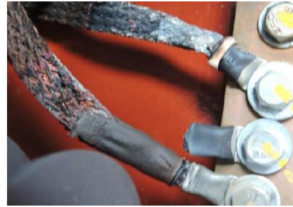
Fig.17. Shield burnt by high current circulation
