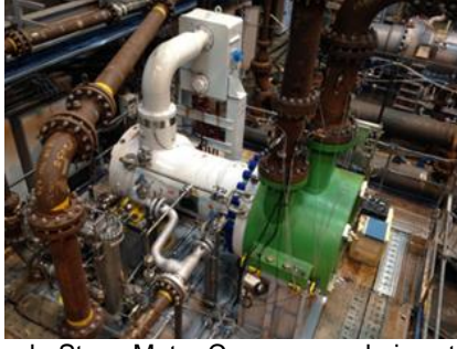
Fig.6. Single-Stage Motor-Compressor during string test
