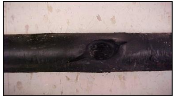
Fig. 3 Cable failure after DC HIPOT and prior to off-line 50/60Hz PD test
