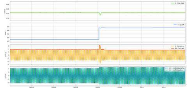
Fig 16. Output voltage reference adjusted from 85% to 100% by a step variation. Motor speed at 1600rpm under 55% of load.
