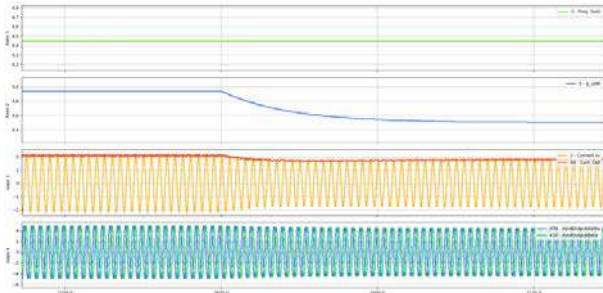
Fig 13. Output voltage reference adjusted from 100% to 90%, with low pass filter. Motor speed at 1600rpm without load.
