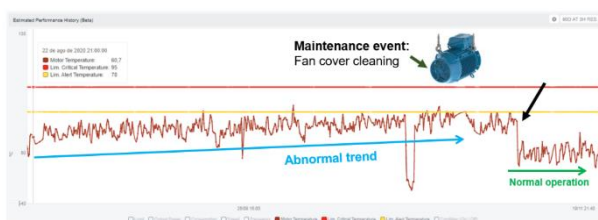
Fig. 7 Overheating occurrence and detection
