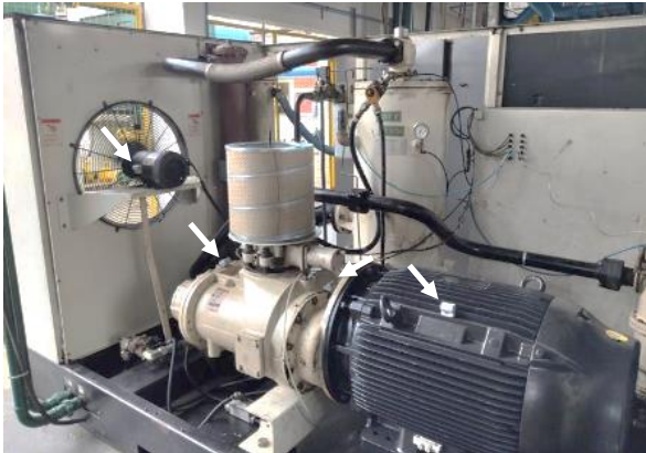
Fig. 16 Air compressor with 150kW electric motor with online monitoring via four wireless sensors
