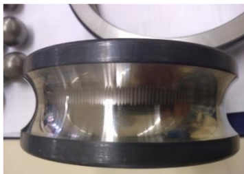
Fig. 17 Detail of damaged bearing (inner race)
