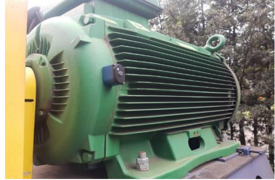
Fig. 10 Online monitoring of 315kW fan electric motor
