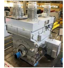
Fig.28. 16MW@8000 rpm 2-pole induction motor on AMB(s).
