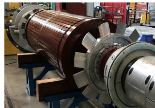
Fig.18. 2-pole Induction Rotor.
