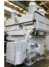
Fig.28. 16MW@8000 rpm 2-pole induction motor on AMB(s).
