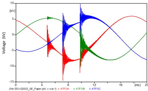
Fig. 16 Case 1: Voltage at the primary side of FCMA autotransformer
