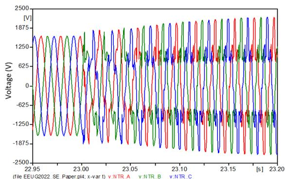
Fig. 12 Zoom on voltage at neutral point - simulation
