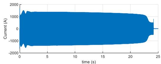
Fig. 8 Current passing through SS-CB – On-site measurement
