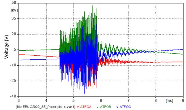
Fig. 18 Case 2: Voltage at the primary side of FCMA autotransformer
