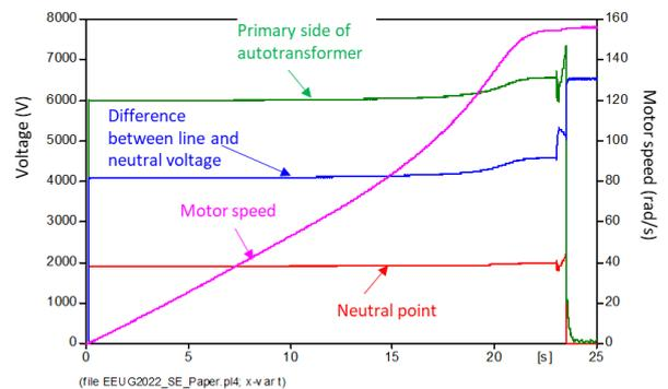
Fig. 13 Evolution of voltage at different point in the system during motor starting
