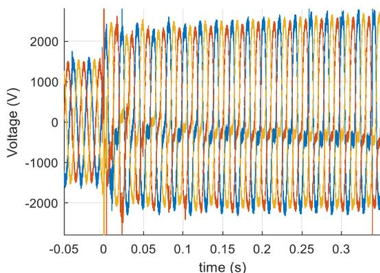
Fig. 11 Zoom on voltage at neutral point - measurement
