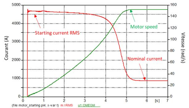
Fig. 2 Motor starting with ideal voltage source
