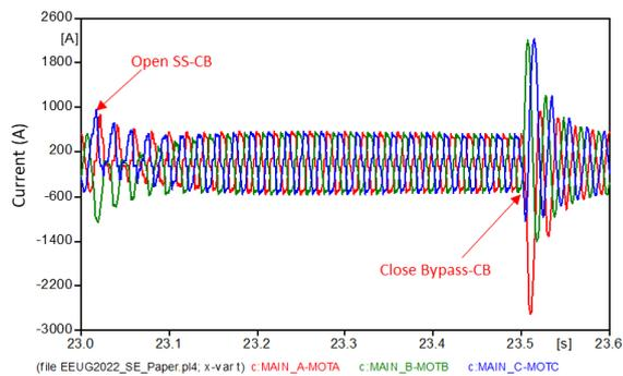
Fig. 10 Zoom on the current in motor - simulation
