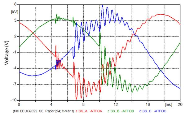
Fig. 19 Voltage at the primary side of FCMA autotransformer with presence of RC snubber
