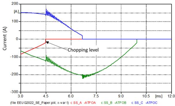
Fig. 15 Case 1: Current passing through SS-CB at opening
