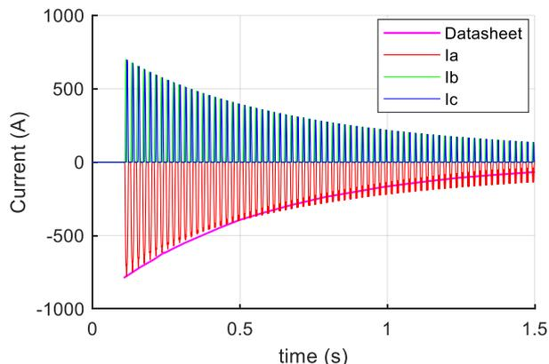
Simulation of the transformer energization
