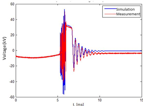
Fig. 5 Model of VCB – simulation vs. tests results
