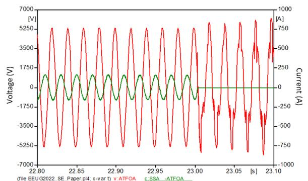
Fig. 14 Zoom on current passing through SS-CB at opening
