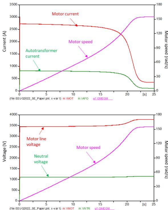
Fig. 6 Current and Voltage rms values in FCMA system during motor starting
