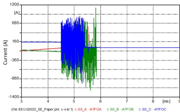
Fig. 17 Case 2: Current passing through SS-CB at opening
