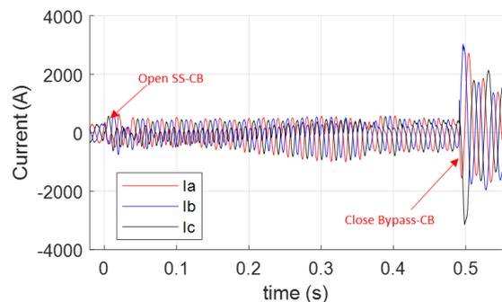
Fig. 9 Zoom on the current in motor - measurement
