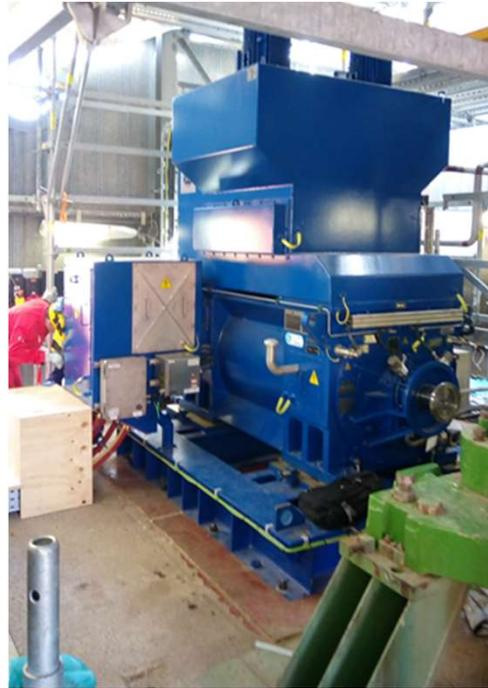
5.7 MW @ 6 400 rpm on Oil bearings
