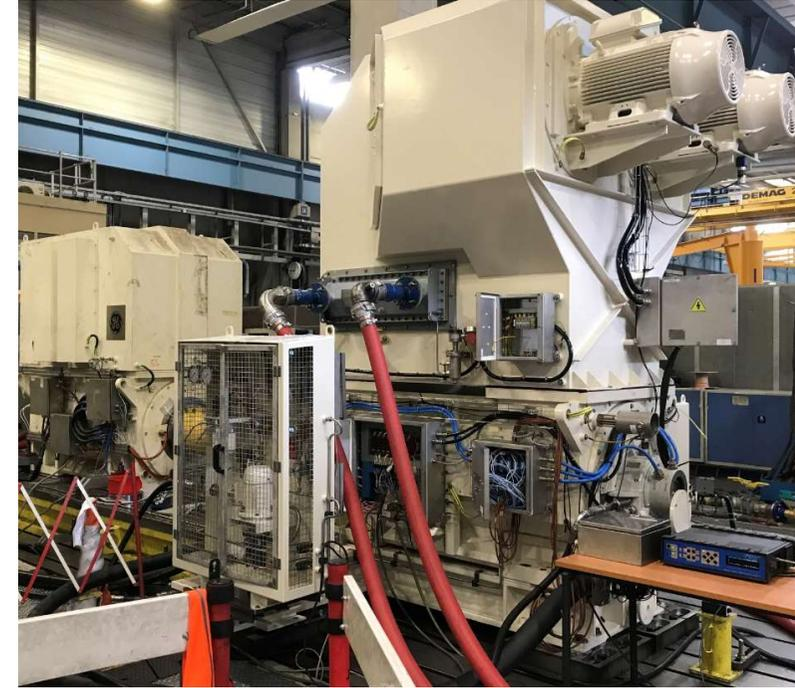
4.9 MW @ 4 900 – 7 500rpm on Oil bearings
