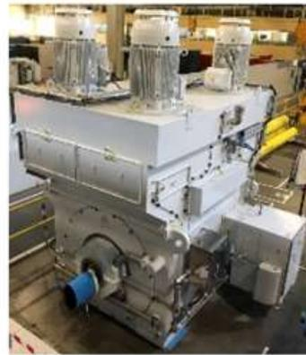
High-speed induction motor on AMB(s) brings substantial reduction in weight and footprint reducing the size of the topside structure of the offshore platform
