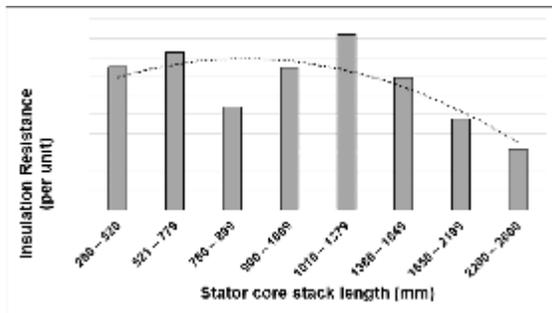
Fig. 5 IR value versus stator core stack length
