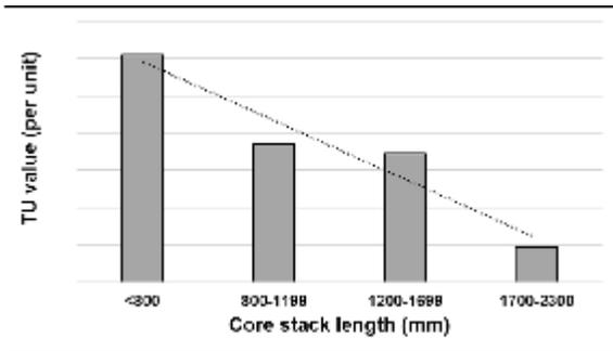
Fig. 11 TU value as core stack length increases
