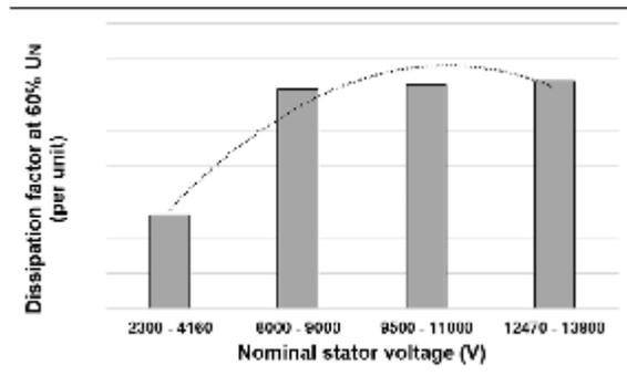
Fig. 7 TD value at 60%  $U_N$  as nominal stator voltage increases
