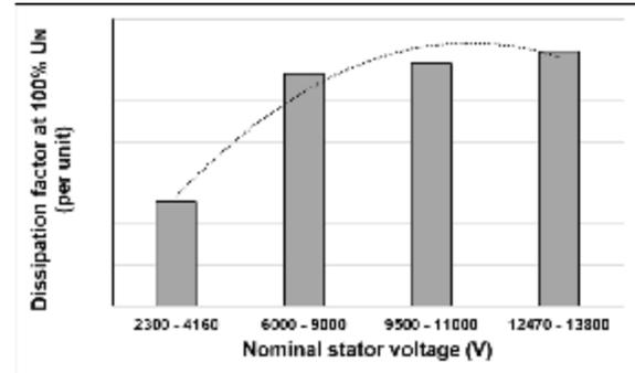
Fig. 8 TD value at 100%  $U_N$  as nominal stator voltage increases
