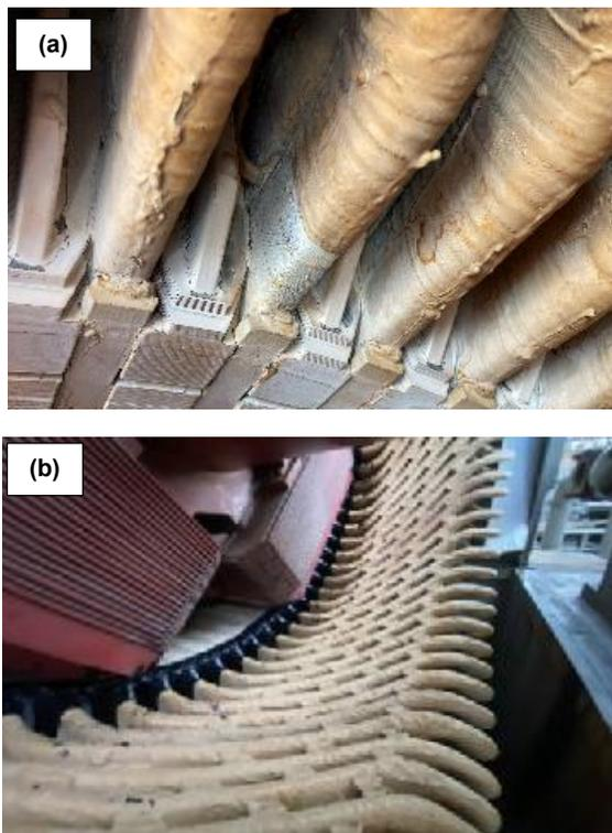
Fig. 15 Stator winding (a) before and (b) after remedial work
