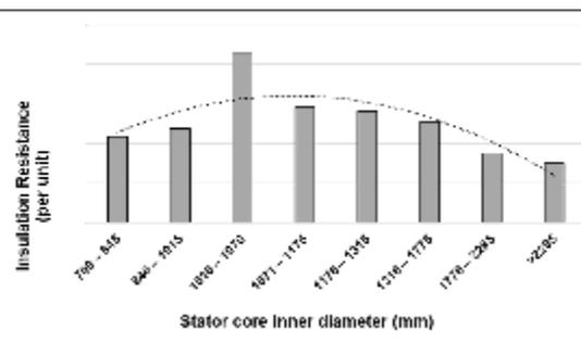
Fig. 3 IR value with regards to stator core inner diameter
