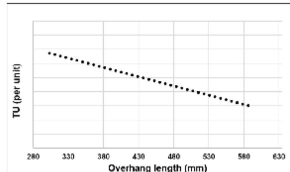
Fig. 10 TU value as overhang length increases
