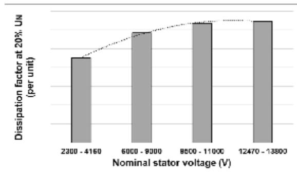
Fig. 6 TD value at 20%  $U_N$  as rated stator voltage increases
