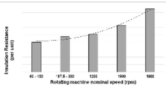
Fig. 2 IR value as machine nominal rated speed increases.
