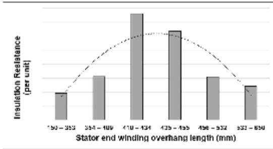
Fig. 4 IR value versus stator endwinding overhang
