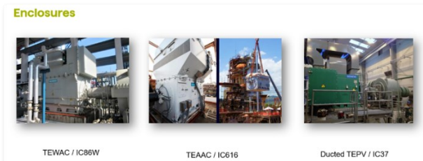
Fig.16 Different possible cooling types for High Speed motors
