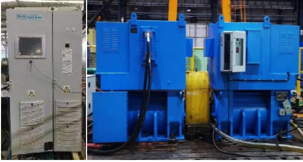
Fig. 7 Coupled PMSM motors for test (active magnetic bearing control and motor on the left, sleeve bearing motor on the right)
