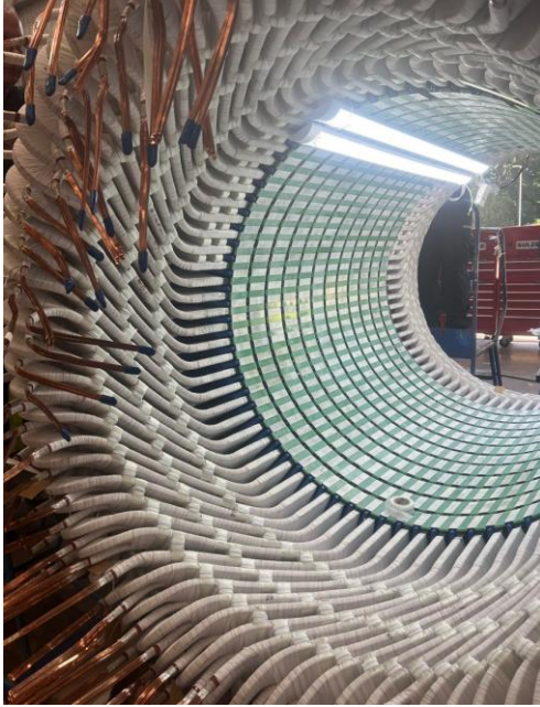
Fig. 3 HV winding showing coil leads
