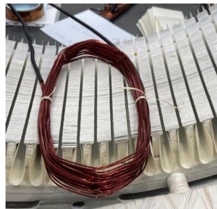
Fig. 2 LV coil showing slot liners in place
