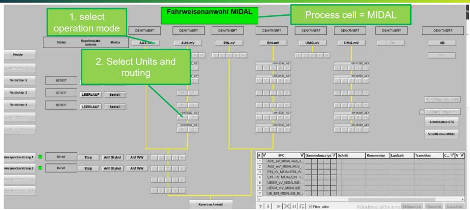
The sequence of selection does not represent the gas flow direction
