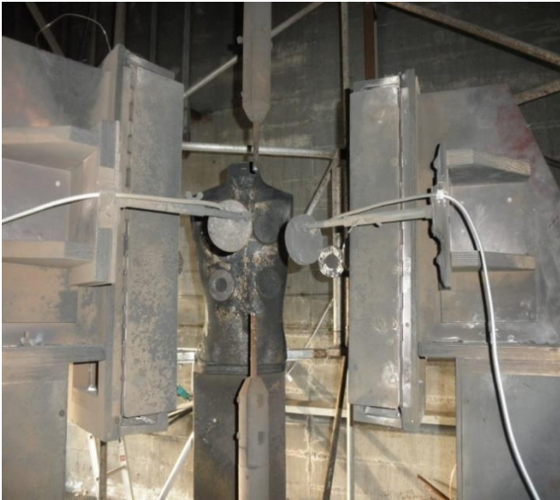
Fig. 2 – Open Arc Test Apparatus.
