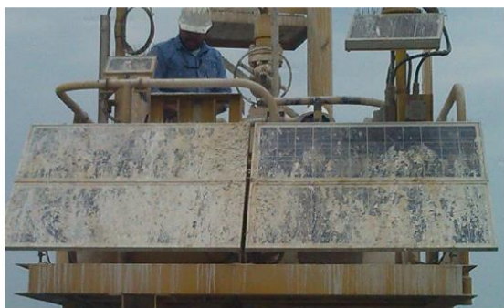
Figure 3: Existing soiled PV solar panels
