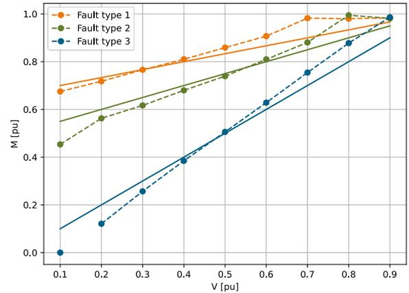
Figure 13: Available torque for different voltage dips
