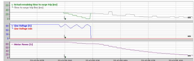
Figure 21: {2-phase, 60 ms, 74 %} voltage dip, starting with 30 ms time to STL, hence, the drive trips.
