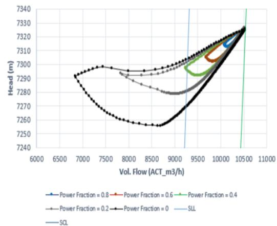
Figure 16: Compressor transient responses. 200 ms voltage dip, for variable residual power (0, 0.2, 0.4, 0.6, 0.8). Aspen Hysys Dynamics simulation study.
