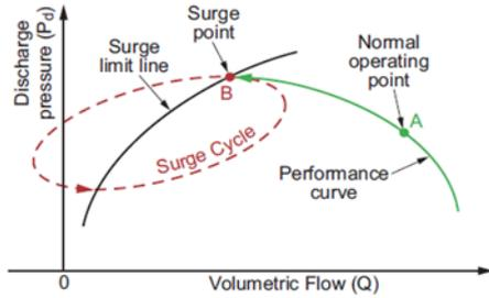
Figure 2: Compressor operation curve
