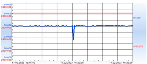
Figure 19: Voltage dip scenario ride-through with eLVRT.
