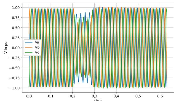
Figure 8: Voltage measured at PCC during a grid fault event.
