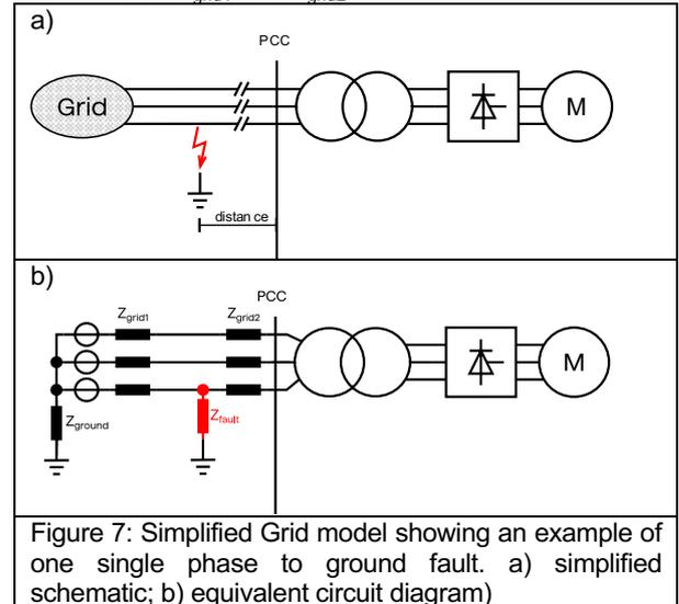
Figure 7: Simplified Grid model showing an example of one single phase to ground fault. a) simplified schematic; b) equivalent circuit diagram)
