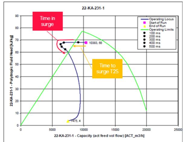
Figure 15: Compressor transient responses. Trip, Time-to-surge and Time-in-surge.
