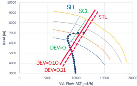
Figure 17: Compressor map and Safe Trip Line. STL = 0.21 was found from the simulation study, while a less conservative limit at STL=0.10 was found during commissioning.
