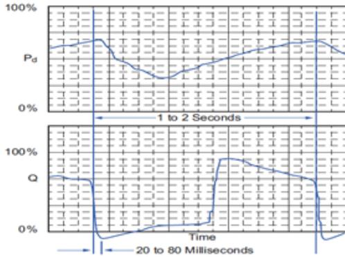
Figure 3: Pressure and flow fluctuations when crossing the surge point shown in Figure 2 (sudden loss of driving torque)
