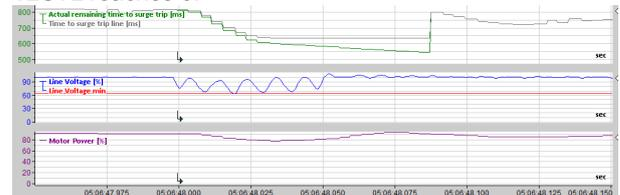
Figure 20: {2-phase, 60 ms, 64 %} voltage dip, starting at safe distance to the STL and ride-through is achieved.
