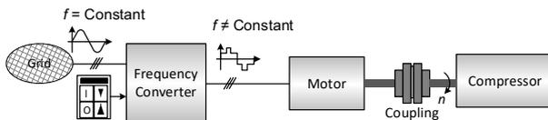
Figure 4: Simplified electrical drive system with VFD
