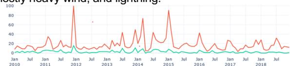
Figure 1: incidents of faults (red) or disconnections (green) per month for power lines 220-420 kV
