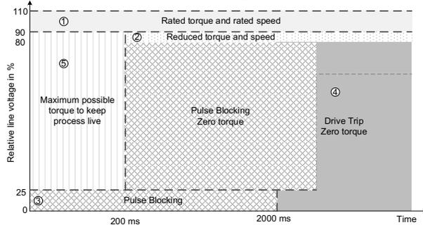
Figure 12: Operating rang during grid faults.
