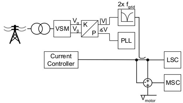
Figure 10: Simplified control logic
