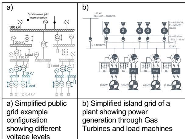
Figure 6: Possible grid configurations
