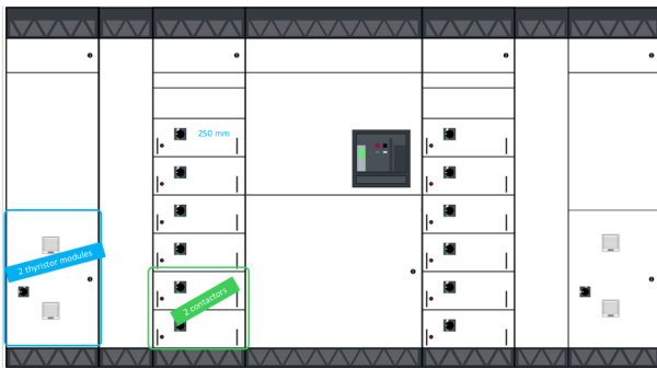
Fig 10: comparison of contactors and thyristors integration in a LV switchboard
