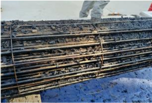
Fig. 3 Effect of Fluid Overtemperature
