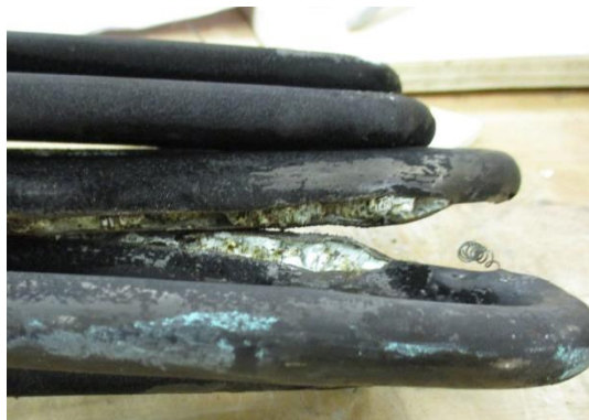
Fig. 5 Failed Electric Heating Elements
