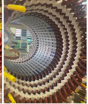
Fig. 2. Prototype after spacers and lashing application.
