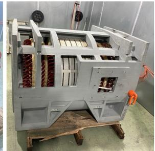
Fig. 11. 13.8 kV prototype stator inside the frame.
