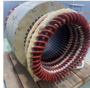
Fig. 10. 13.8 kV prototype stator before frame.
