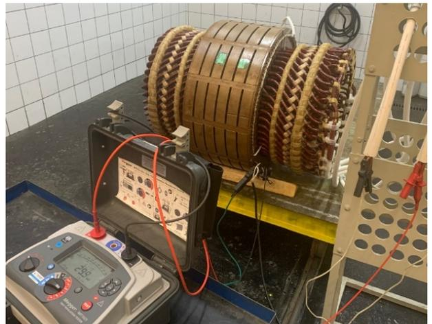
Fig. 3. Initial evaluation of the prototype stator.
