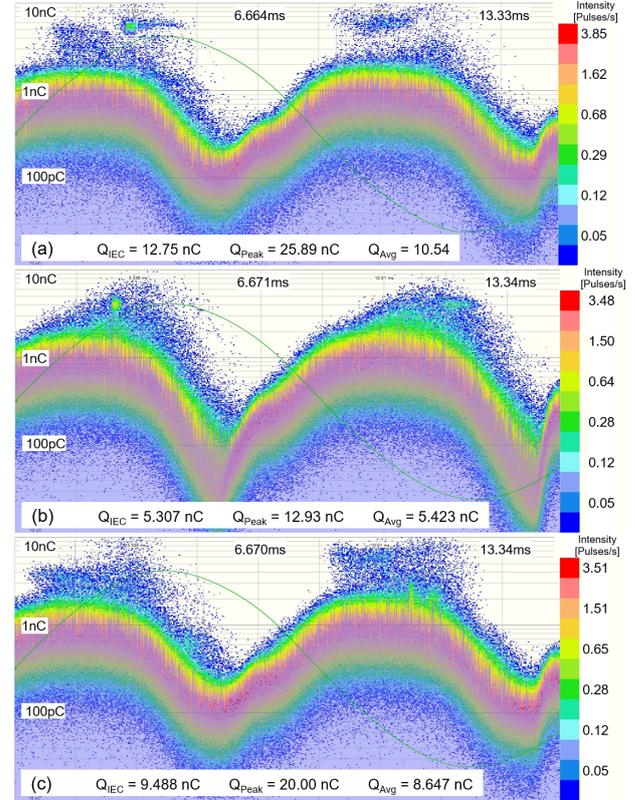
Fig. 6. PD evaluation of the stator after cable routing at 21 kV for (a) Phase U ( $Q_{Peak}$ : 25.89 nC); (b) Phase V ( $Q_{Peak}$ : 12.93 nC); (c) Phase W ( $Q_{Peak}$ : 20.00 nC);
