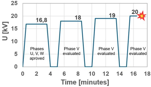
Fig. 7. Voltage scheme applied in the first ignition test of the prototype stator.
