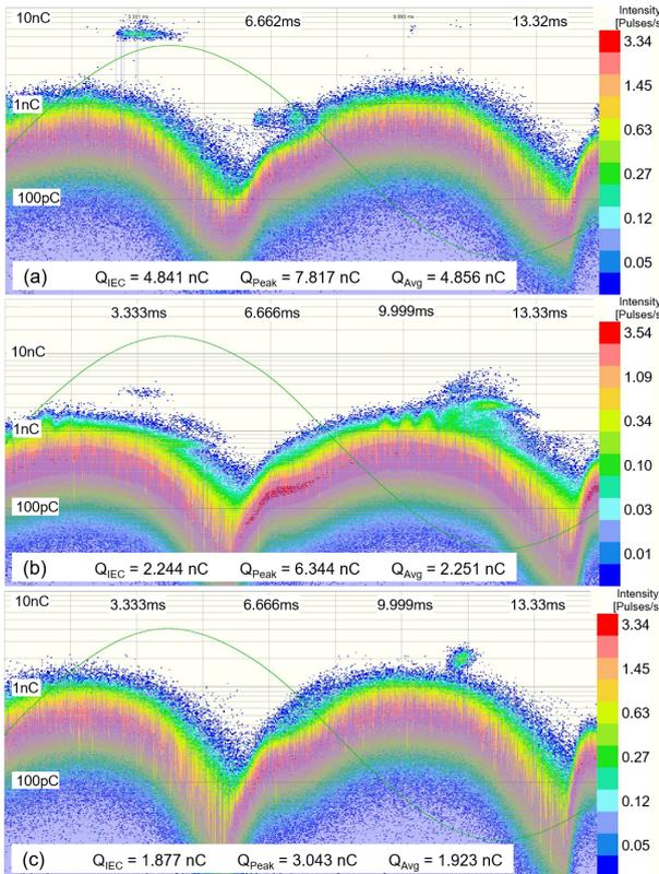
Fig. 5. PD evaluation of the stator before cable routing at 21 kV for (a) Phase U ( $Q_{Peak}$ : 7.817 nC); (b) Phase V ( $Q_{Peak}$ : 6.344 nC); (c) Phase W (Before:  $Q_{Peak}$ : 3.043 nC).
