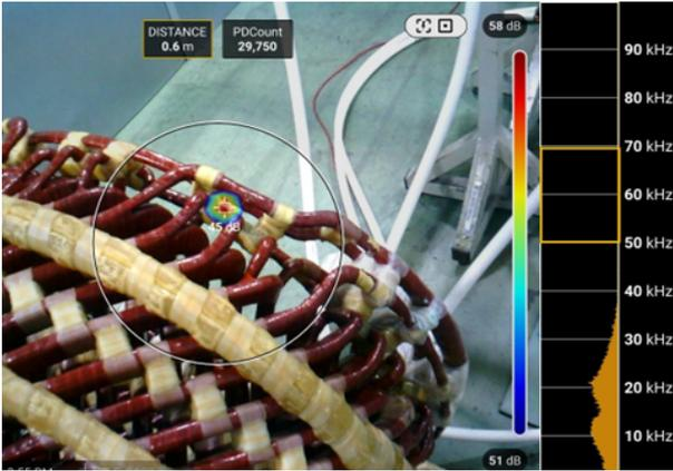
Fig. 4. Imager test example of the prototype stator.
