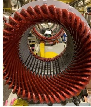
Fig. 1. Prototype before spacers application.
