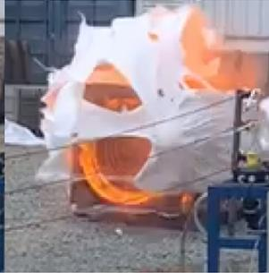
Fig. 9. First prototype stator ignition at 20.0 kV.
