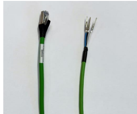
Fig. 4 Ethernet cable with RJ45 connector vs. SPE cable
