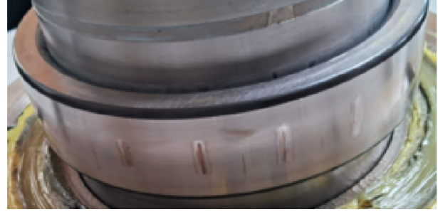
Fig. 7 During inspection, identified BPF1.
