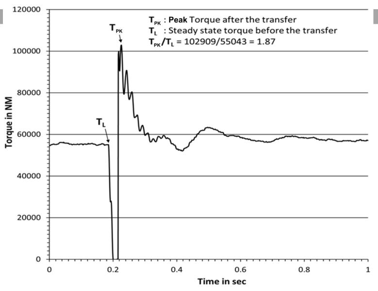
Motor Air Gap Torque, Before and After Transfer PCIC MIDDLE EAST
