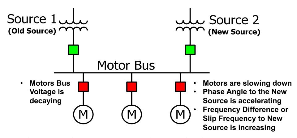
Open Transfer Time = The time from the Old Source Breaker trip to the New Source Breaker close
