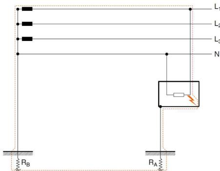
In TT system, there is no protective earth conductor accompanying the phase conductor. In this system, all exposed-conductive-parts and extraneous-conductive-parts of the installation must be connected to a common earth electrode. The impedance of the earth fault loop therefore consists mainly in the two earth electrodes (i.e. the source and local electrodes) in series, so that the magnitude of the earth fault current is generally too small
