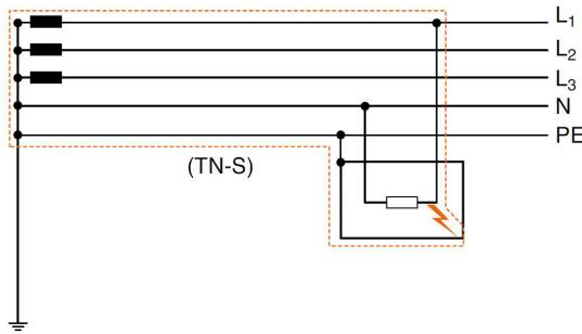
In TN-S system all exposed and extraneous-conductive-parts of the installation are connected directly to the earthed point of the power supply by protective conductors
